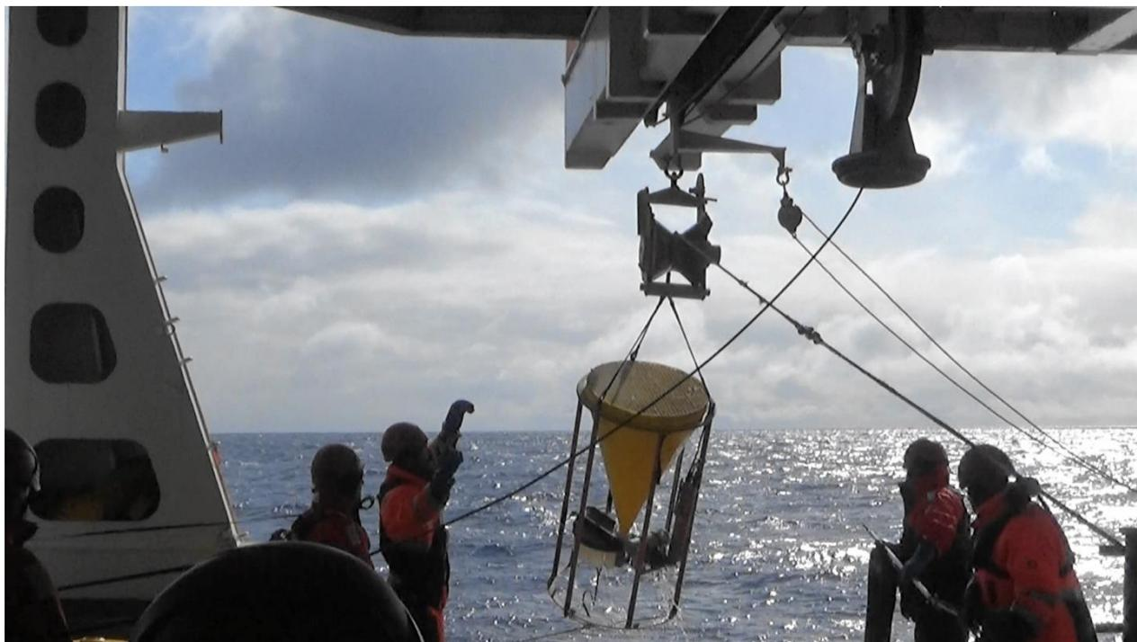
Sediment trap recovering by means of the telescopic boom crane in the sheltered area, B-Deck.
