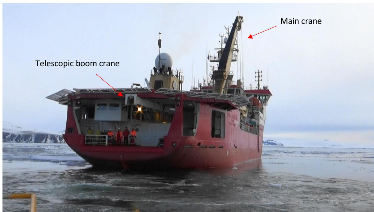
The RV Laura Bassi from the stern. The main Crane is visible on the starboard side. The telescopic boom crane is also visible in the sheltered area.
