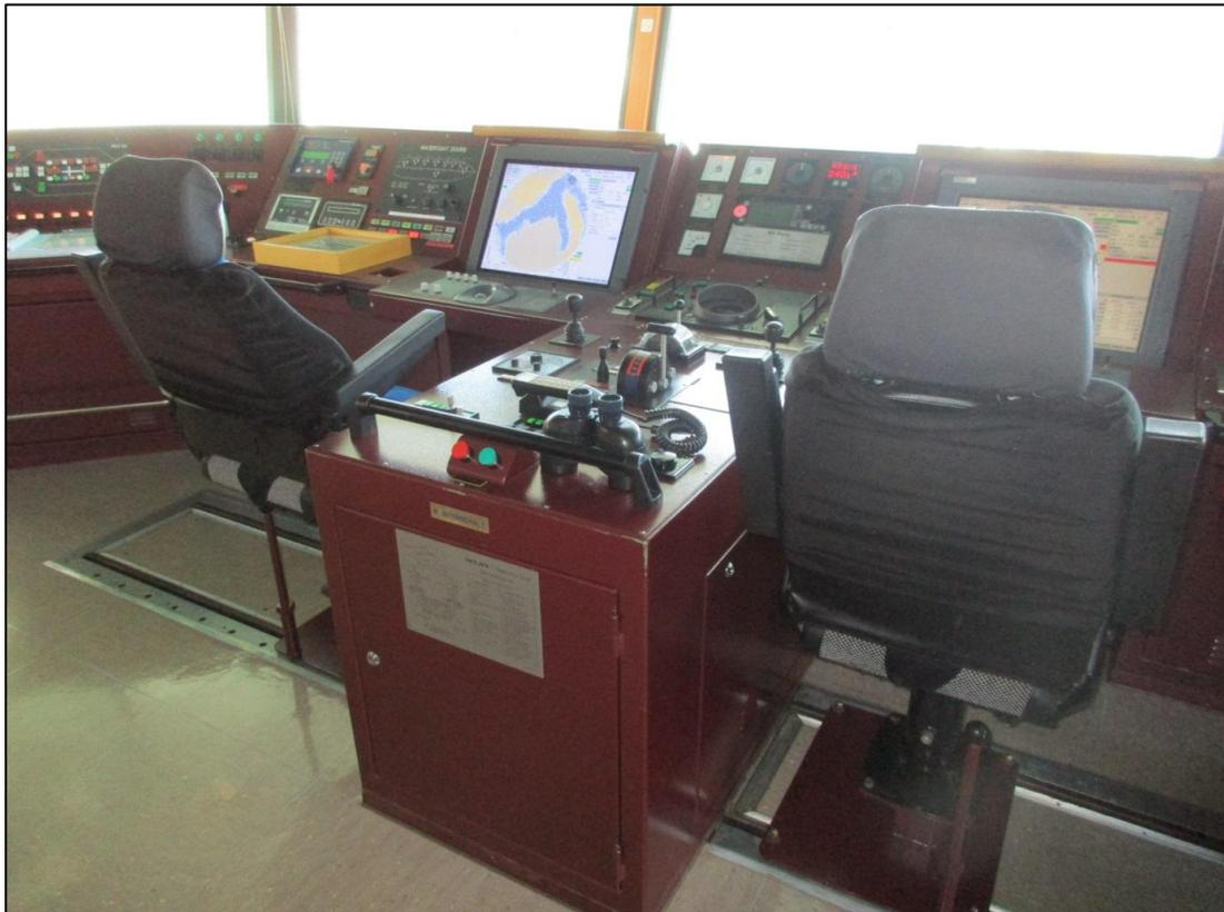
Figure 7: Wheelhouse central console
