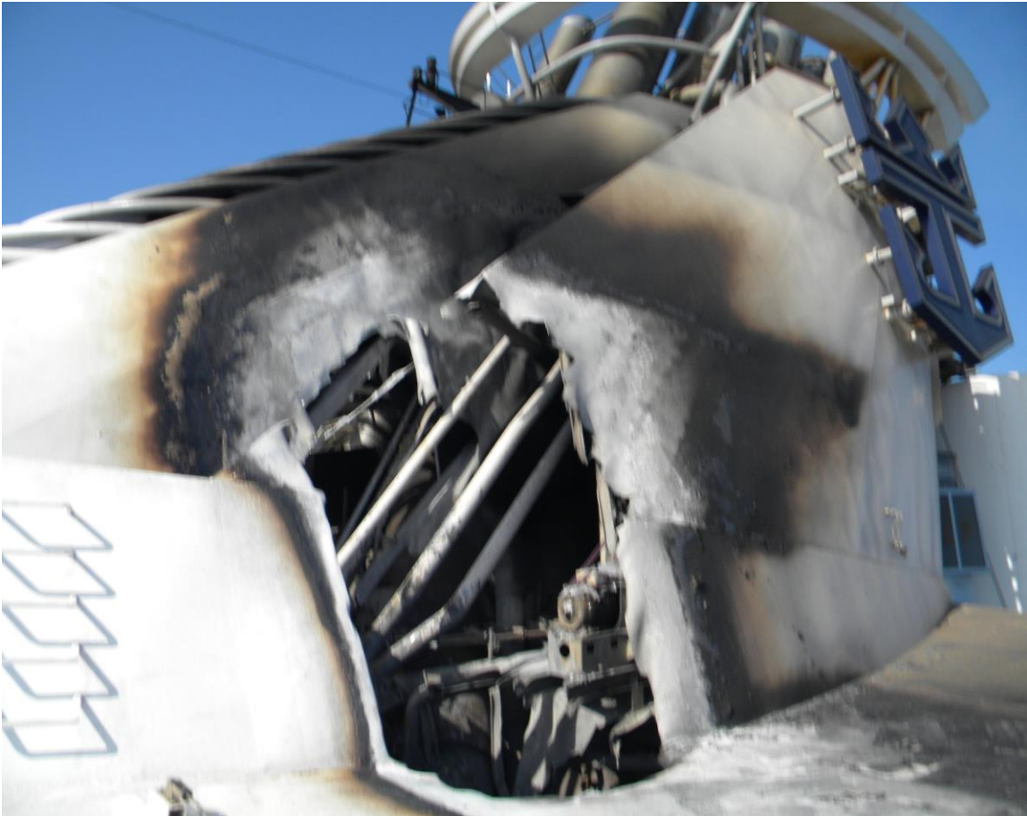
Figure 16: External damage at the Viking Crown, deck 16
