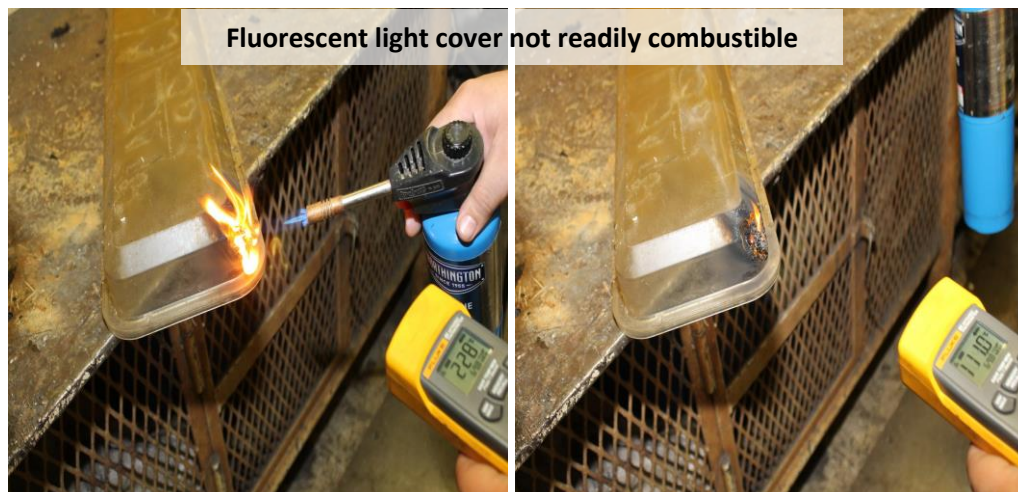
Figure 12: Florescent lighting fire tests
