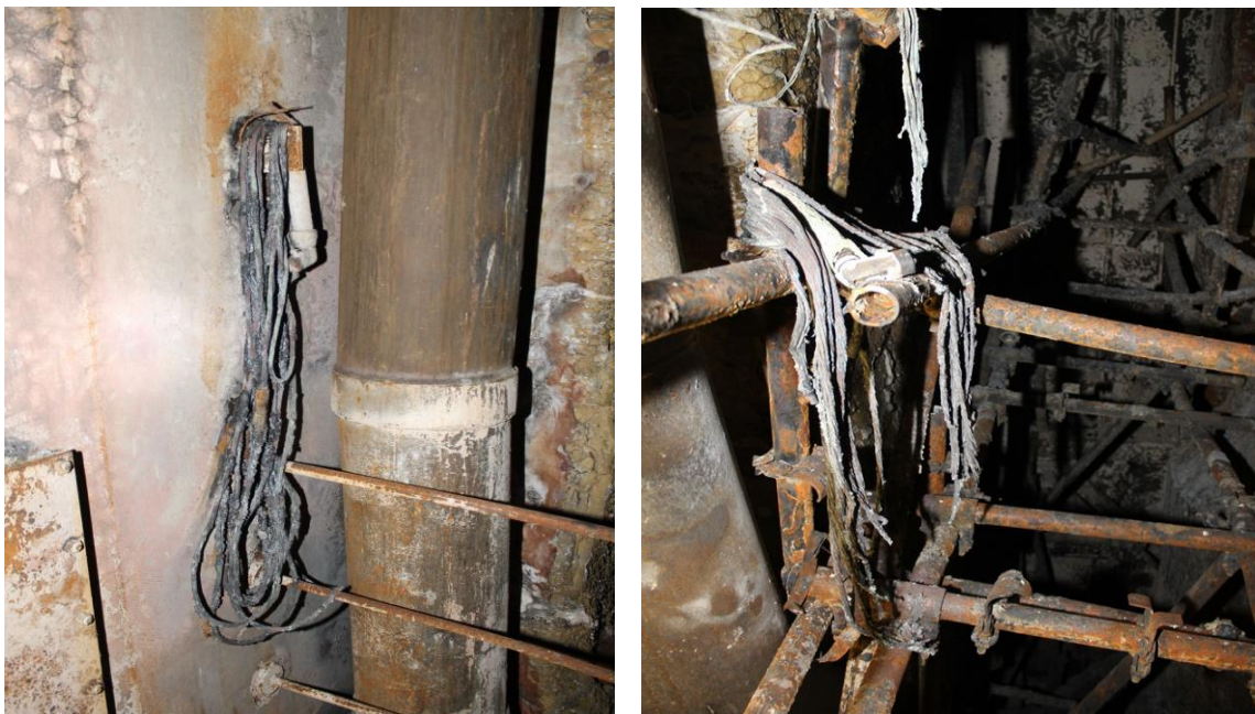
Figure 9: Plasma cutting torch leads pictured after the fire
