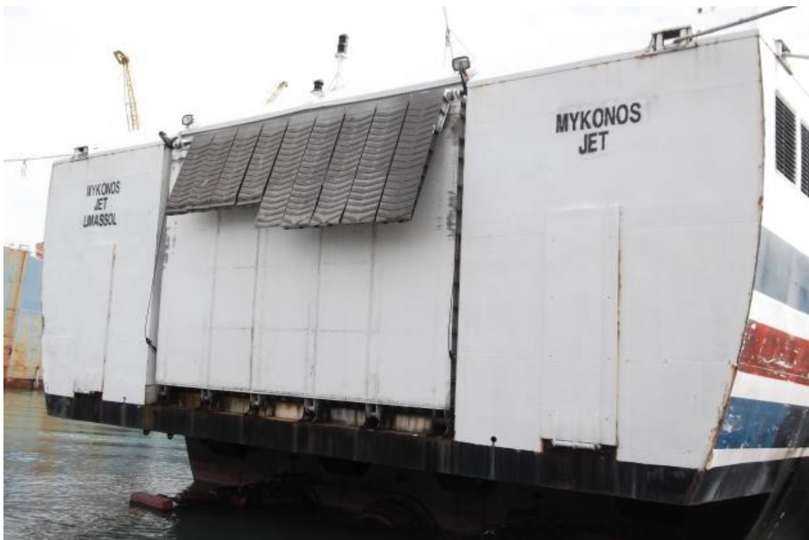
Stern view of HSC “Mykonos Jet”, showing: Port ramp door for passengers, Centre ramp door for vehicles, Starboard ramp door for passengers Class Assessment (for admission to Class): Port of survey MOKPO-South Korea. Date of survey 25/10/2016: - Outside shell plate with doors and steering device have been inspected visually and found in good condition
