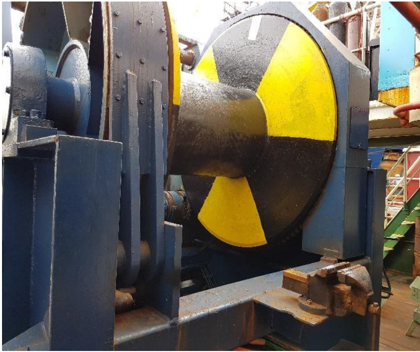
Tug-Boat “Symphony 14” full length of the primary tow wire was released from the wire clamp during sinking of the HSC “Mykonos Jet”
