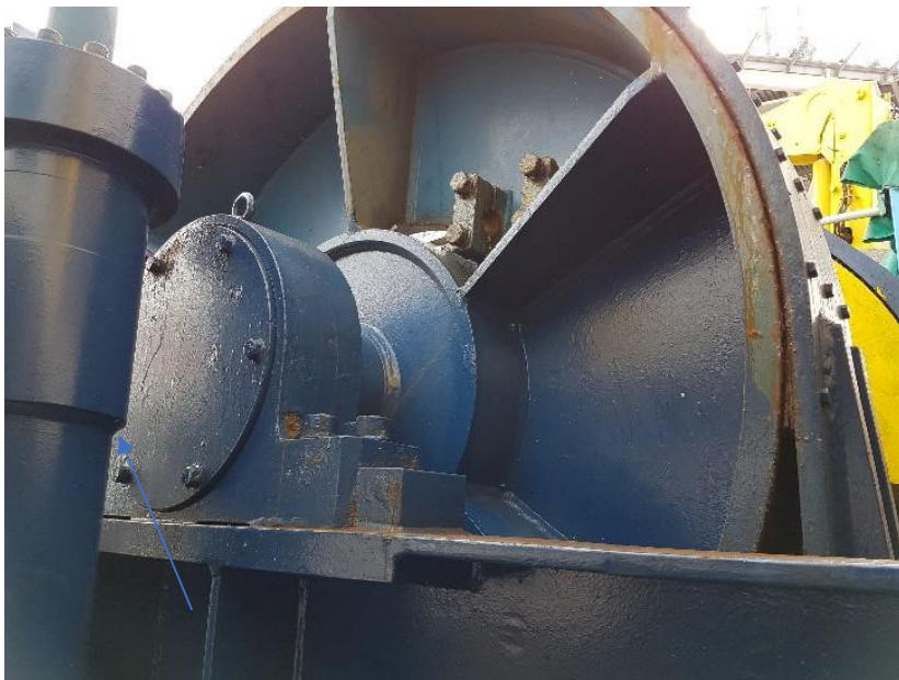
The Wire clamp of the tow wire which was released during the sinking
