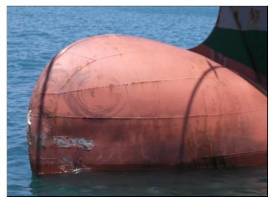
Figure 17: Damage to the bulbous bow
