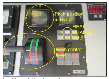
Figure 9: Close view of the port bridge wing console
