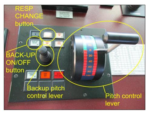
Figure 10: Wheelhouse console showing CPP controls
