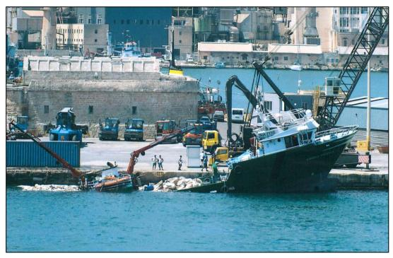
Figure 15: Angela Arcella's massive flooding and loss of reserve buoyancy
