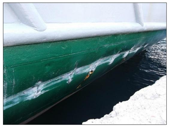
Figure 18: Ship side damage caused by contact with the quay
