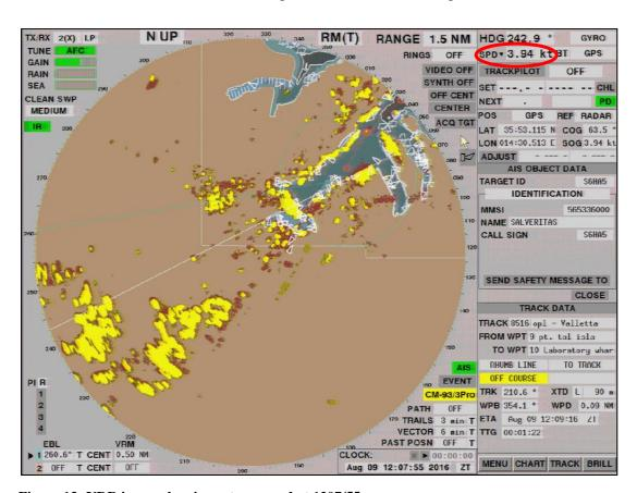
Figure 13: VDR image showing astern speed at 1207/55s
