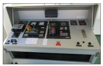
Figure 8: Port bridge wing console
